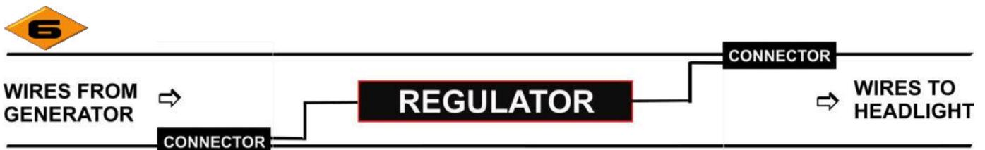
XGEN AND XGEN5 REGULATORS protect all types of bulbs, including Vacuum, Krypton, Halogen, and Nicelite LED dynamo bulbs (regulated 1W white headlight bulbs and 1W red tail light bulbs).
